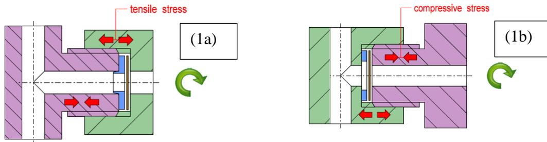
Figure 5: change bad tensile stress (left) to Figure 6 good compressive stress (right)
