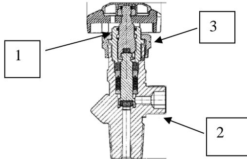
Figure 4: Valve with cover nut
