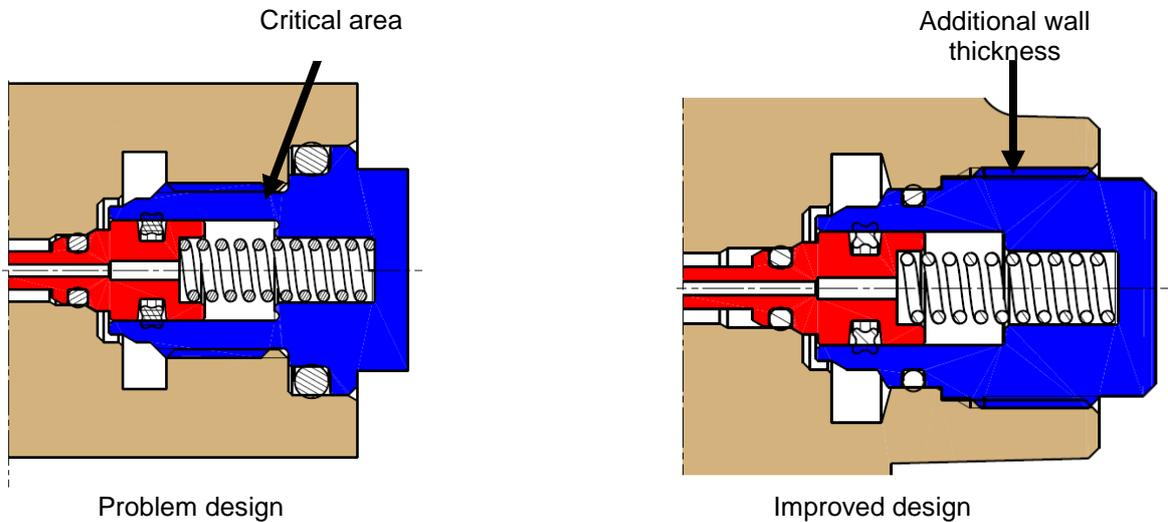
Figure 7: Improved valve design
