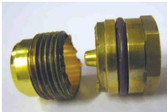
Figure 3: defective residual pressure valve plug
