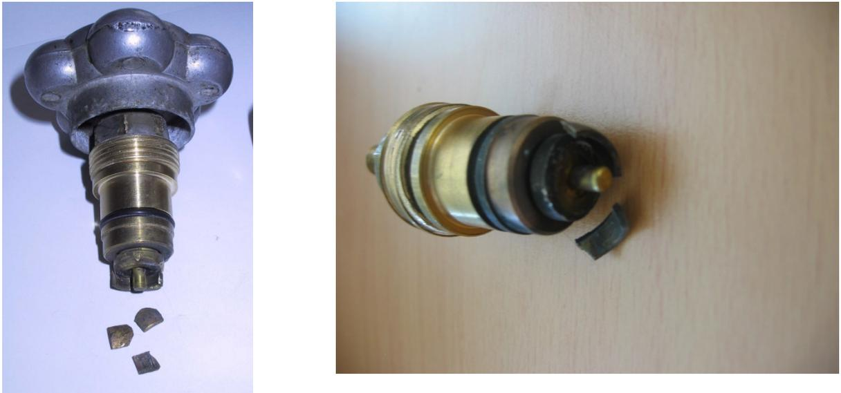
Figure 1: broken lower spindle seal retention skirt
