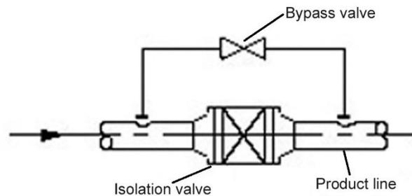
Figure 3—Example for a bypass system
